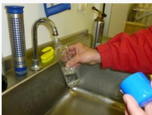
Figure 6 Compliance Officer taking a water sample at the point of compliance (for microbiology) for a Regulated supply
