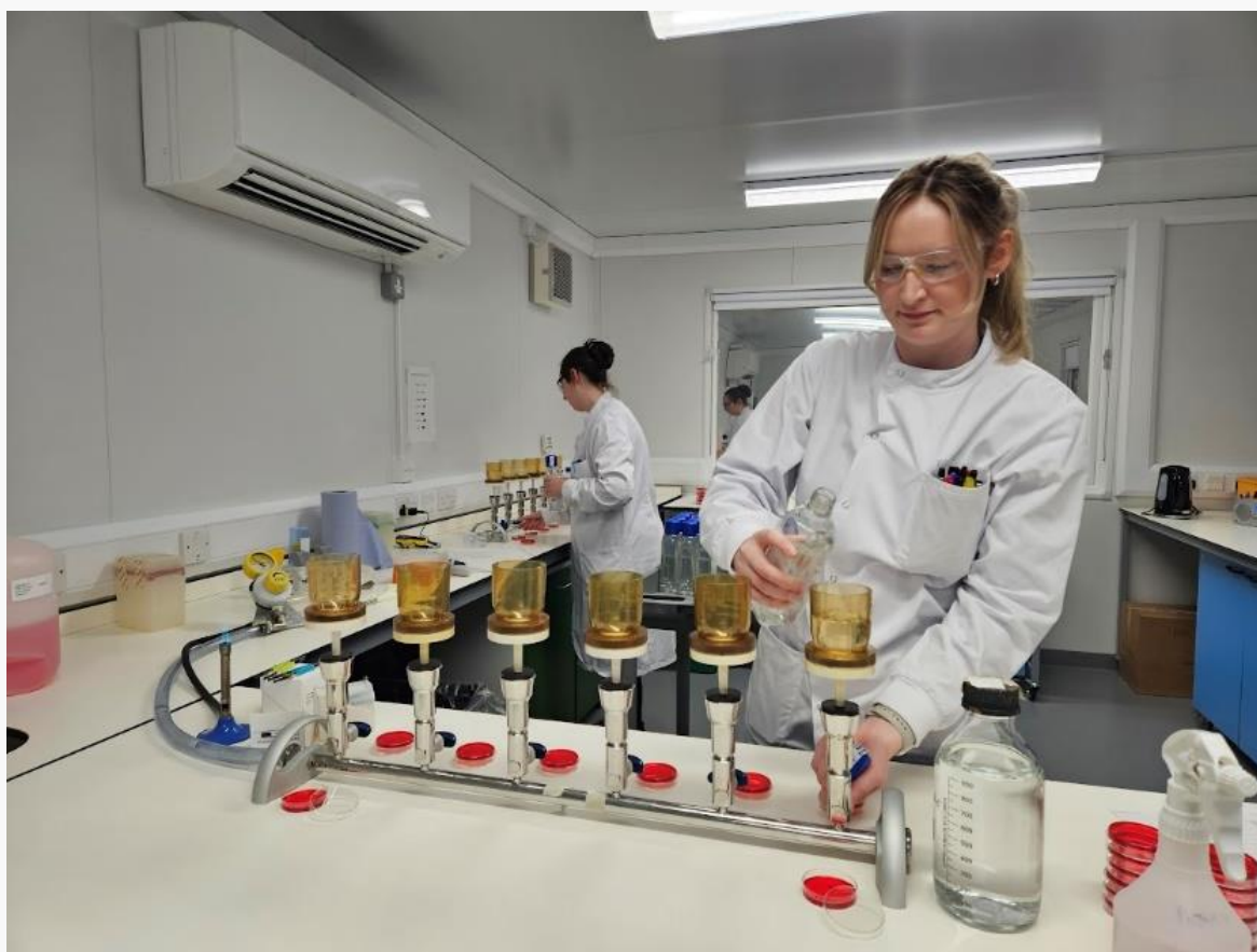
Figure 16 A Scottish Water microbiologist filtering a water sample.
