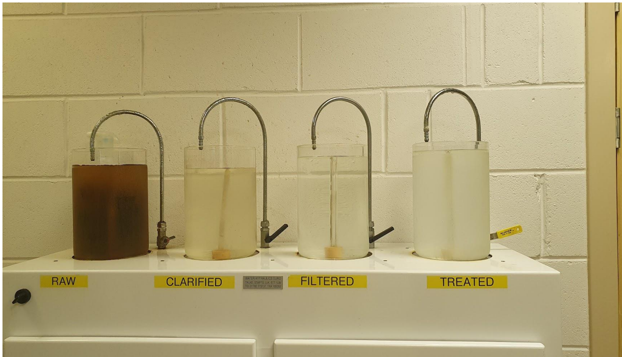
Image 2 Clarity Jars showing water appearance through the processes in a water treatment works
