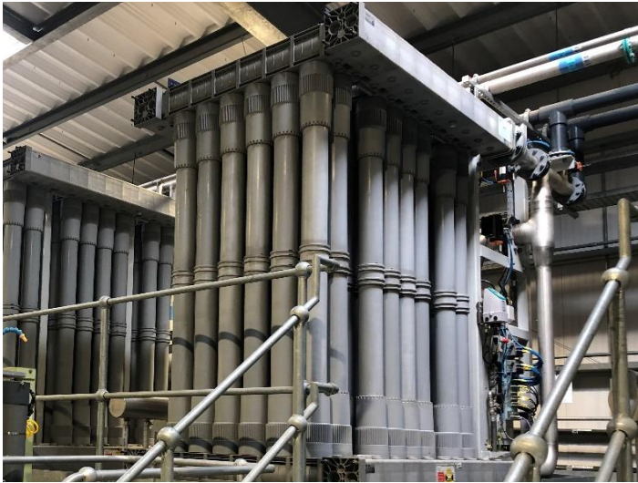
Image 3 A Membrane Treatment Process
