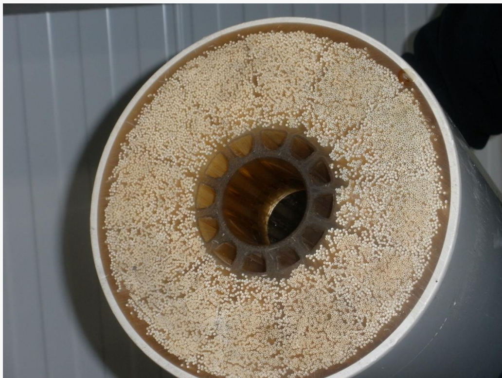
Figure 22 Cross section of a membrane filter at a Scottish Water WTW
