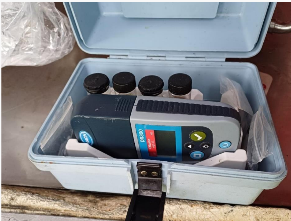
Figure 7 is a chlorine meter to measure the amount of total and free chlorine in a water sample
