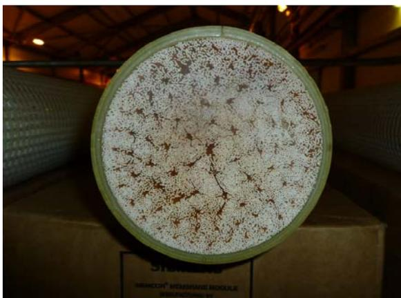
*Hollow fibre membrane used at Invercarnie WTW (end on). The membrane is composed of many hollow fibres, like drinking straws. These are submerged in the water to be treated and this is sucked through the walls into the membrane straw, filtering it. Clean permeate water is pumped out of the end of each hollow fibre.*
