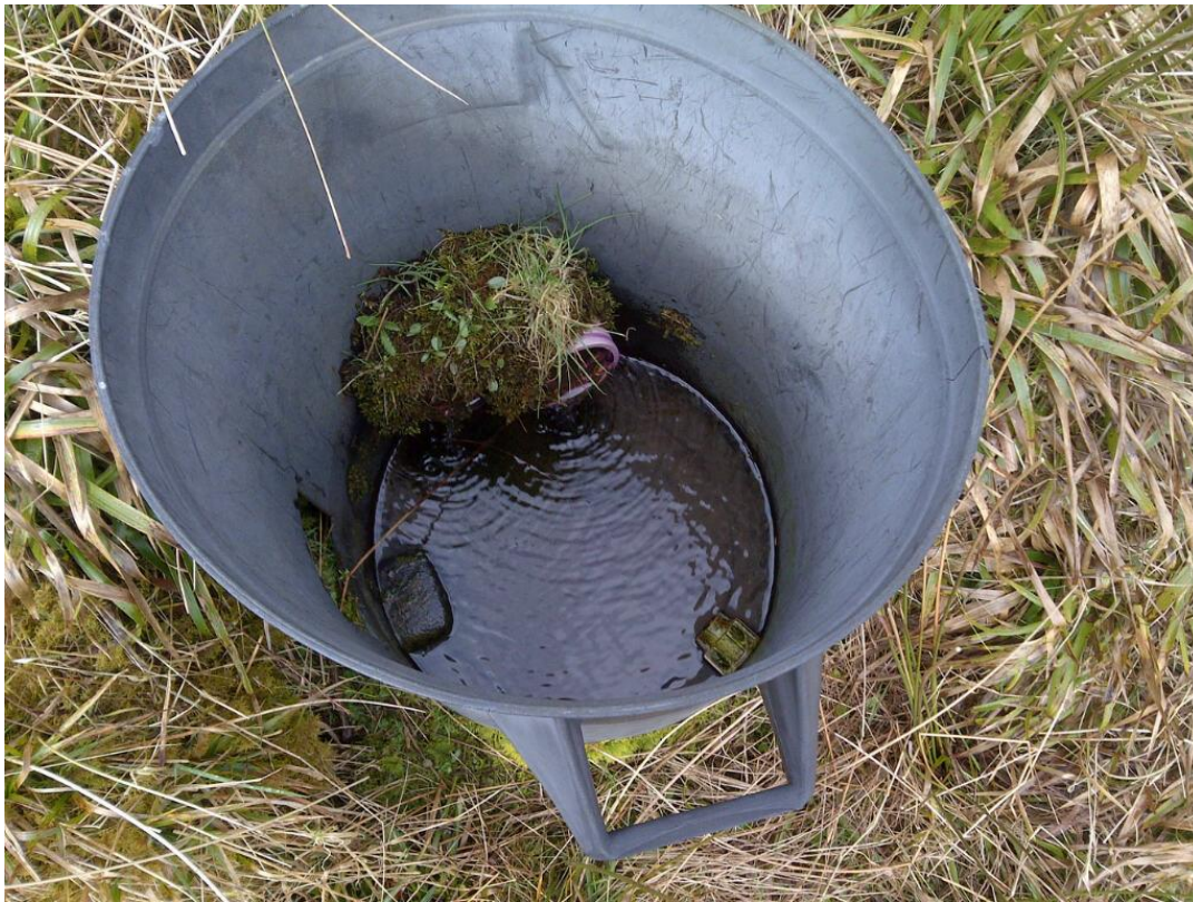
A Dustbin Used as a Crude Collection Device
